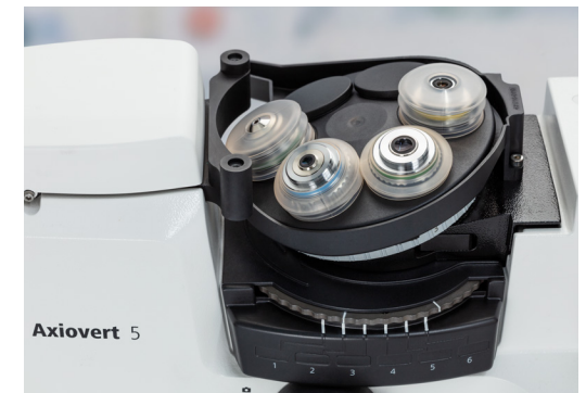
The Aqua Stop II protects the objectives and other optical components inside the microscope from liquids.
