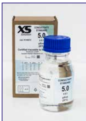
Conductivity standard 5 µS/cm with NIST traceability
