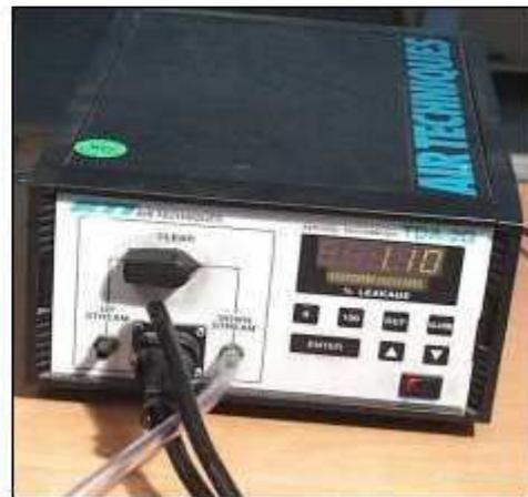
**Figure 5.** Wrong result: filter leaking
