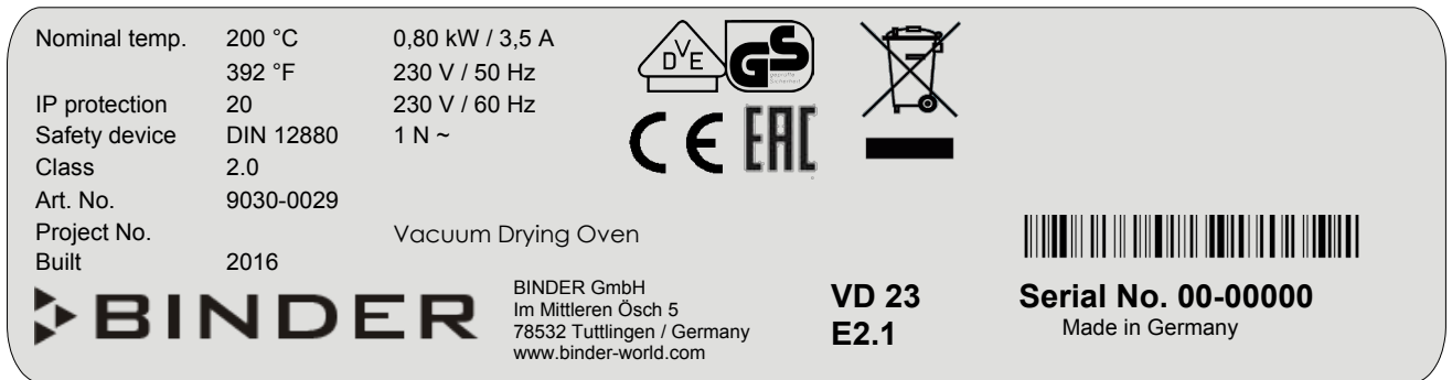
Figure 2: Plaque signalétique (exemple VD 23 standard)
