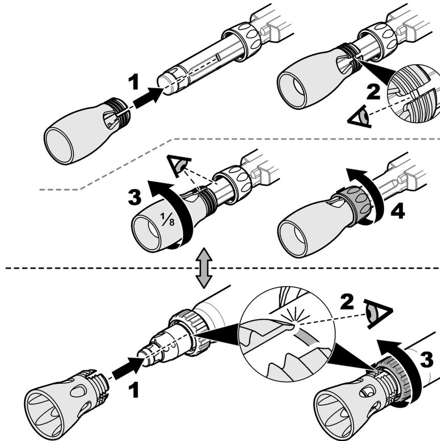
**EN:** Make sure that the cover of the pressure sensor module is fully seated to keep out water or damage to the probe may occur.
