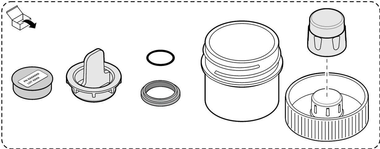
**EN:** Replace the sensor cap and iButton® at the same time. The iButton® updates the probe calibration for the new sensor cap.
