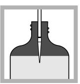
8. Use a TenSette Pipet to add 0.1 mL of the chlorine solution to Bottle #1 while stirring. Put the end of the pipet tip under the water to dispense the chlorine. To prevent highly localized areas of chlorine concentration is mandatory to stir the sample while the chlorine is added.
