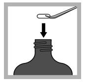
**5.** Use tweezers or tongs to put a stir bar magnet into each bottle. Do not touch the stir bar.
