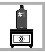
**6.** Put Bottle #1 on the stir plate. Set a low stir speed. A small vortex will show on the surface of the liquid.
