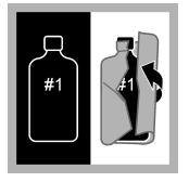
**13.** Put the sample bottle in a dark location or wrap with foil.
