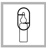
**7.** Use the ampule breaker to open a Chlorine Dosing Solution Ampule.
