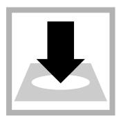
13. Within 5 minutes after the timer expires, insert the prepared sample into the cell holder. Point the diamond mark on the sample cell toward the keypad.
