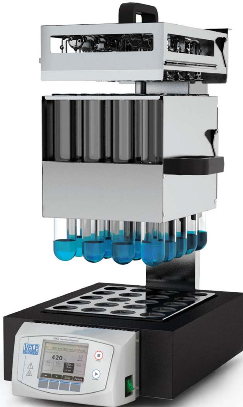
The digester is a widely used instrument in laboratories performing analysis for diversified applications in food&feed, beverage (nitrogen, protein, Total Kjeldahl Nitrogen), environmental (COD, Total Kjeldahl Nitrogen), chemical and pharmaceutical (organic nitrogen) industries. DKL digesters work in accordance with a variety of Standards (such as AOAC, ISO, EPA, DIN etc.).
