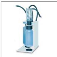
“SMS” Unit is designed for the neutralization of toxic and corrosive fumes coming from oxidative mineralization or other processes.
